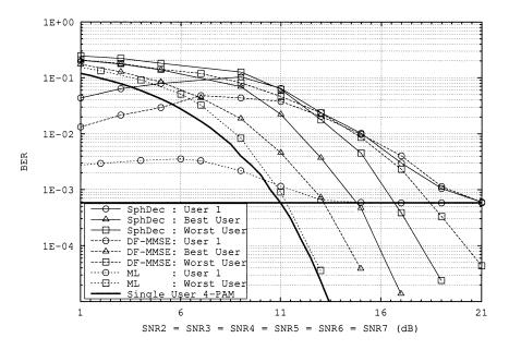
Fig. 8. Asynchronous system: seven users, 4-PAM modulation, SNR1 = 11 dB.
