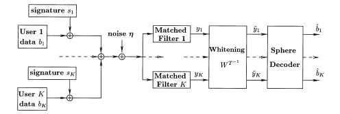
Fig. 2. CDMA system model with joint lattice detection.
