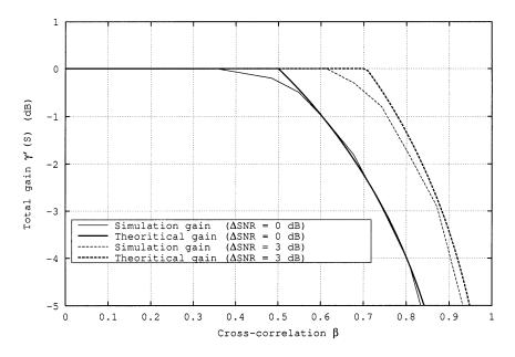
Fig. 9. Synchronous system gain: two users, 16-PAM modulation.
