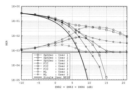
Fig. 7. Asynchronous system: four users, BPSK modulation, SNR1 = 7 dB, three iterations for PIC hard detector.
