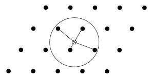
Fig. 1. Geometrical representation of the sphere-decoding algorithm.
