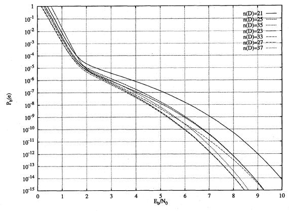
Fig. 7. Bit error probability bounds for rate 1/3 PCCC with interleaving length N = 100 employing as CC the 16-state encoders yielding the value of  $z_{min}$  of Theorem 2.
