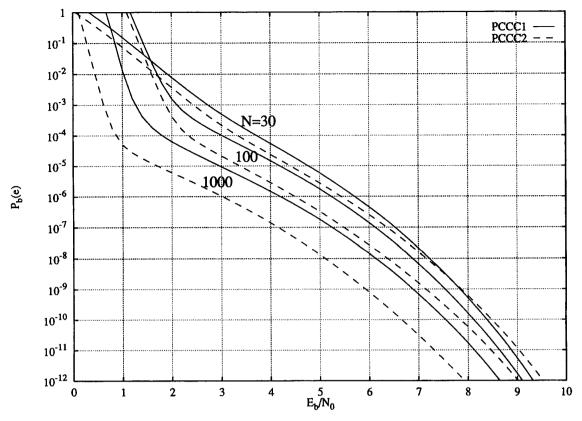
Fig. 3. Bit error probability bounds for PCCC1 and PCCC2 of Example 1 for interleaver lengths N = 30, 100, and 1000.
