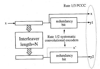
Fig. 1. Encoder structure of a PCCC.
