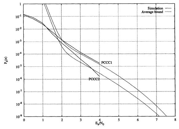
Fig. 5. Simulation results for the codes PCCC1 and PCCC2 (solid lines) compared to ML upper bounds. The simulated suboptimum iterative decoding algorithm used at most 20 iterations.
