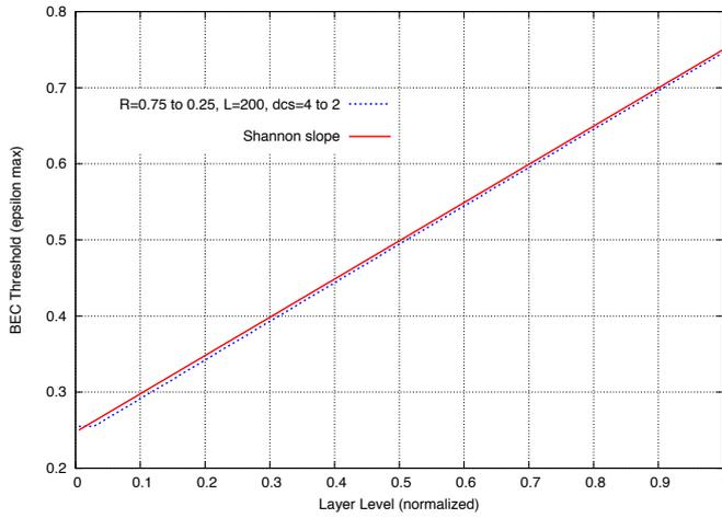
Figure 6. BEC thresholds for a non-uniform chain of forward spatial coupling with  $\aleph = L$  local ensembles varying with the spatial position. Parameters are  $L = 200$ ,  $d_b = 3$ ,  $d_c = 12$  to 4, Rate = 0.75 to 0.25.
