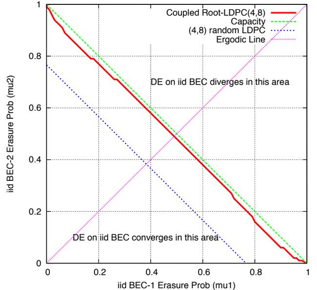
Figure 10. Saturation of the threshold boundary after coupling parity bits. Threshold boundaries for random (4,8)-LDPC and coupled (4,8) root-LDPC ensembles are shown in the erasure plane.
