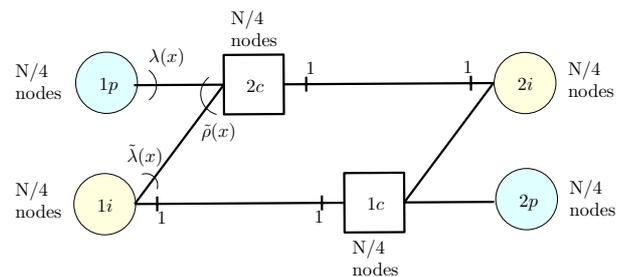
Figure 1. Compact Tanner graph representation for a rate-1/2 root-LDPC ensemble. If the bits transmitted on one fading are erased, the erased information bits are recovered.
