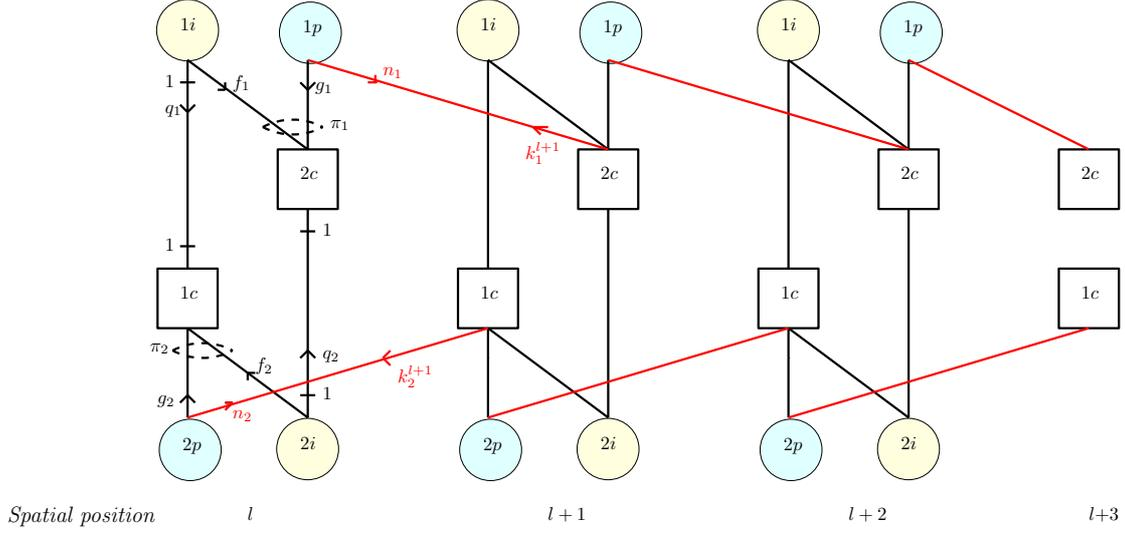
Figure 3. Forward layered spatial coupling of root-LDPC. The chain is terminated at the right end by the checks placed at the spatial position  $L + 1$ . Since only the parity bits are coupled to the checks, this is a partial coupling scheme.
