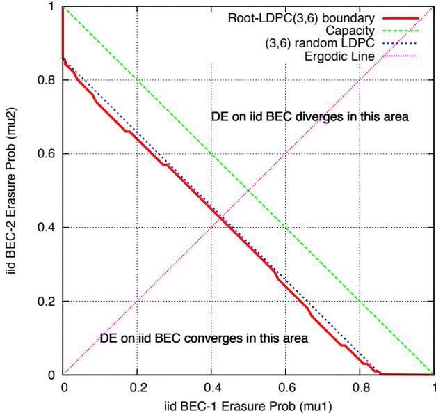
Figure 9. BEC threshold boundaries for random (3,6)-LDPC and uncoupled (3,6) root-LDPC ensembles in the erasure plane.
