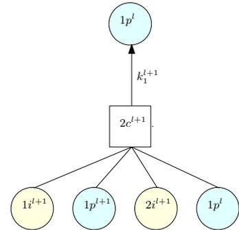
Figure 4. Local tree neighbourhood of checknode  $2c$ . This tree is used to determine the evolution of the backward coupling message  $k_1^{l+1}$ .
