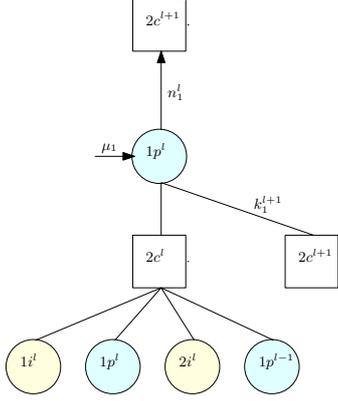
Figure 5. Local tree neighbourhood of bitnode  $1p$ . This tree is used to determine the evolution of the forward coupling message  $n_1^l$ .
