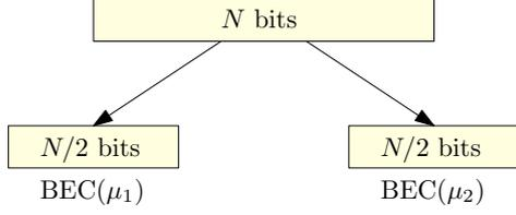
Figure 2. Parallel binary erasure channels where half of the bits are transmitted through  $\text{BEC}(\mu_1)$  and the other half of the bits are transmitted through  $\text{BEC}(\mu_2)$ .
