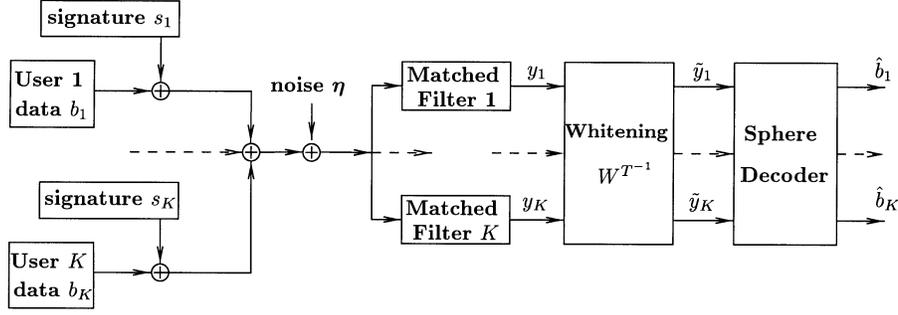
Fig. 2. CDMA system model with joint lattice detection.
