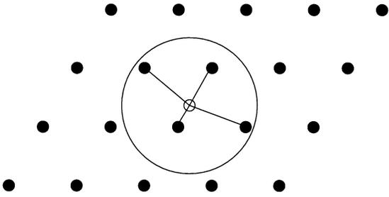
Fig. 1. Geometrical representation of the sphere-decoding algorithm.
