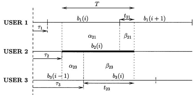
Fig. 3. Asynchronous multiple-access system with three users: interference on user 2.
