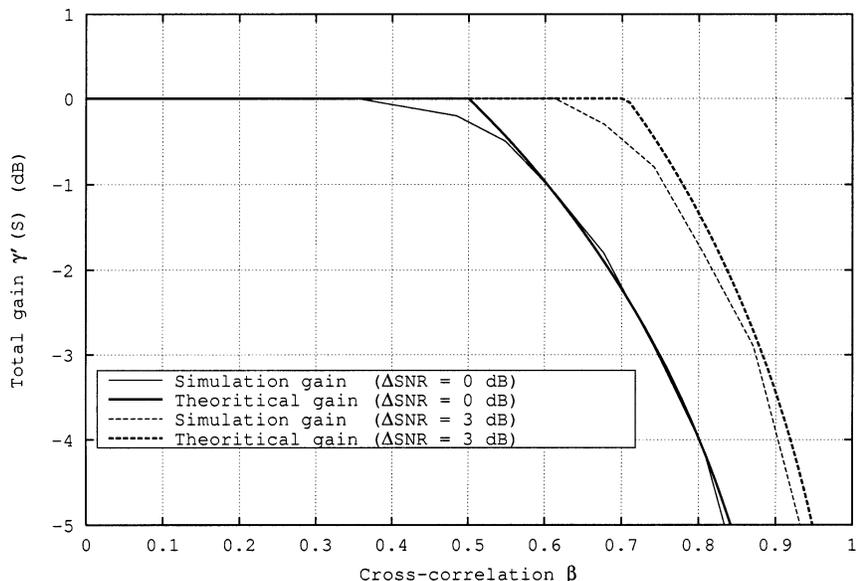
Fig. 9. Synchronous system gain: two users, 16-PAM modulation.
